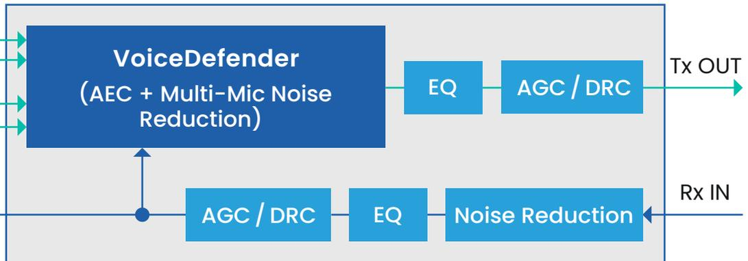
VoiceDefender employs adaptive directional beamforming on 4 microphone signals (2 per ear). A combination of end-fire and broadside beamforming is used to create a single enhanced output, providing a personal zone of voice preservation even in noisy environments.
